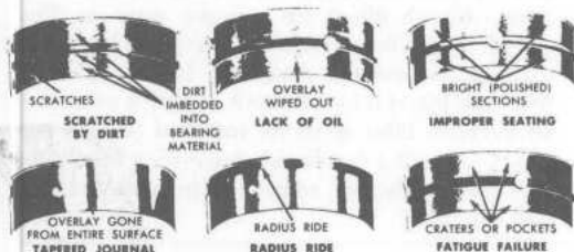
Causes of bearing failure
