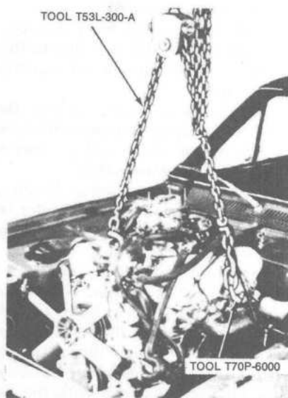
Removing or installing engine—V6 shown
