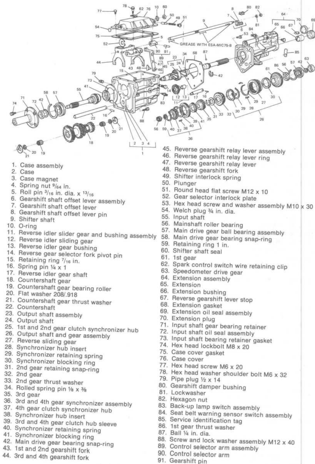
Exploded view—4-speed transmission
