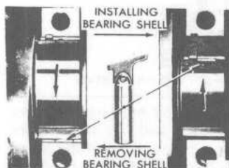
Removal and installation of upper bearing insert using a roll-out pin (© Buick Div. G.M. Corp.)
