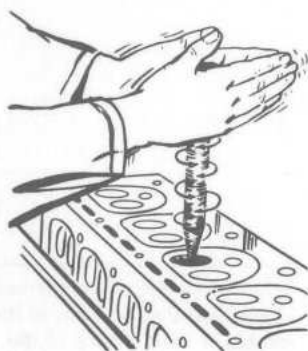
Hand lapping the valves
