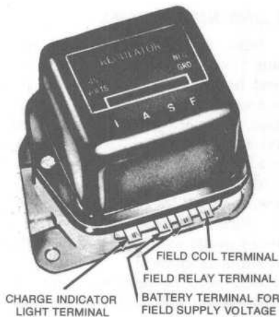
Electro-mechanical regulator terminals
