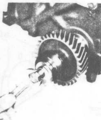
Installing crankshaft gear—2800cc V6
