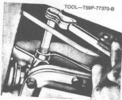
Adjusting low-reverse band (C4 only)
