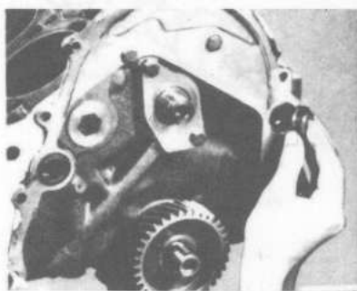
Removing or installing guide sleeves—2800cc V6
