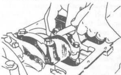
Checking connecting rod side clearance
