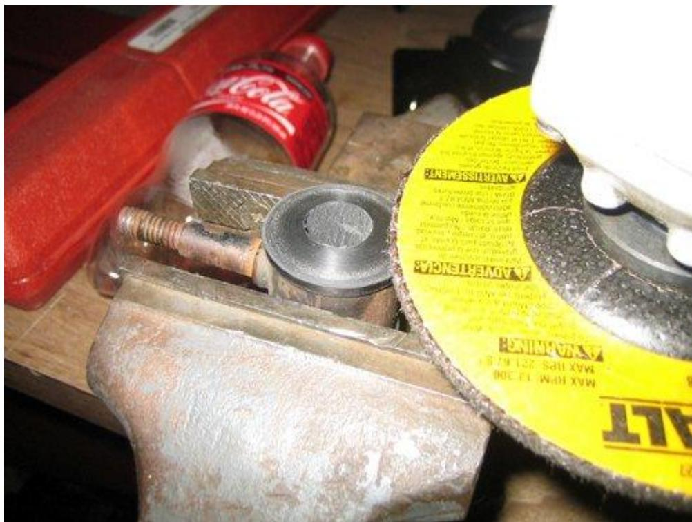
The head of the shackle bushings purchased from Espo is shaped to fit the shackles so it has a slight dome on the head end. This dome needs to be removed so that when the bushings are installed in the metal shell, the width of the assembled end link should be about 1-5/16", not including the inner sleeve. This will allow the teeth on the inner sleeve to stick out a bit from the bushings and "bite" into the end link bracket when installed on the car. Repeat 3 more times.
