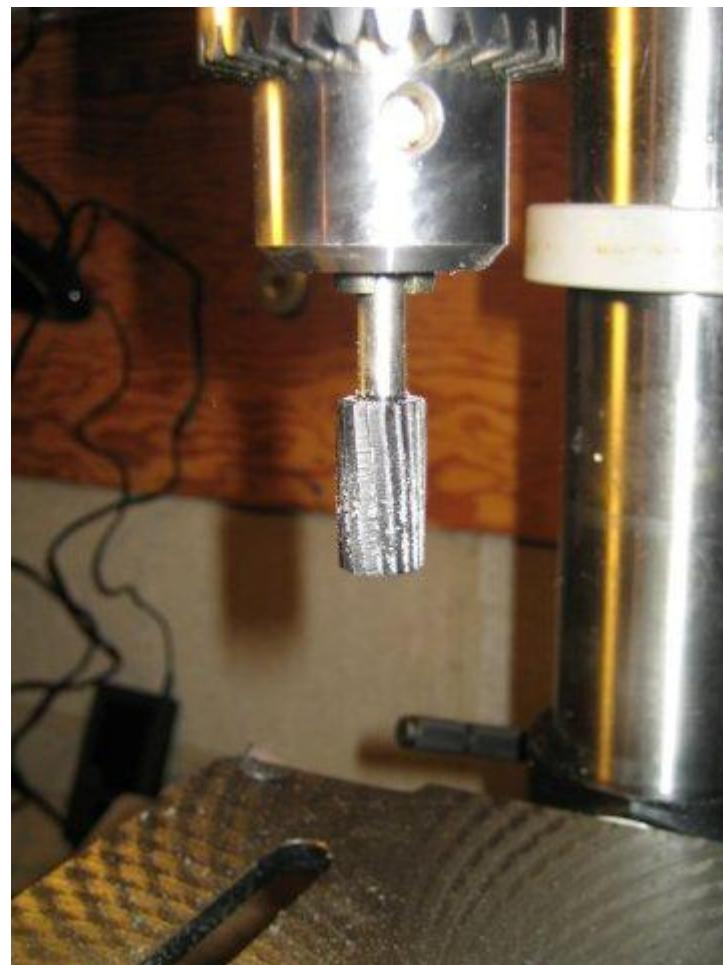
I put a glove on the hand holding the bushing and rotated the bushing against the bit pushing slightly on the bushing.
