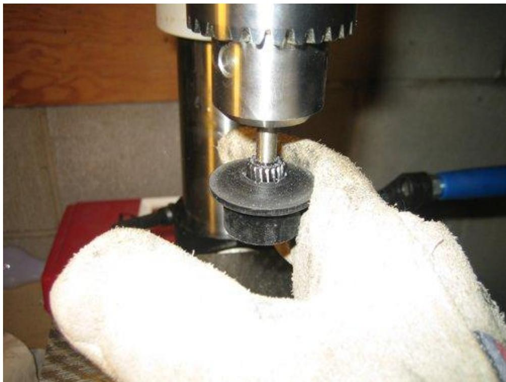
This worked well and slowly increased the diameter of the hole until I was satisfied with the size (should be about 21/32"). The inner sleeve should fit so snuggly that you have to force it in. Repeat 3 more times.
