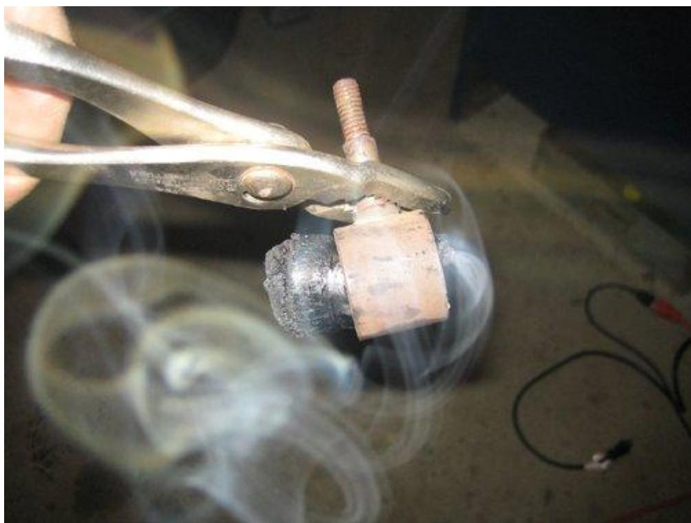
The rubber will expand and soften so that the inner sleeve and rubber can be removed from the outer shell. Use a pair of pliers to hold the bushing and another to pull the inner sleeve out. Remove the rubber. Don't burn yourself!
