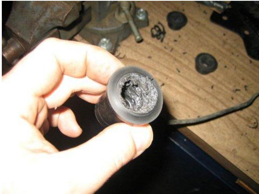
The method that worked best for me with both the drill and the drill press was to get a 1/2" diameter rotary file (Vermont American PN 16677). It just fits inside of the existing bushing hole.
