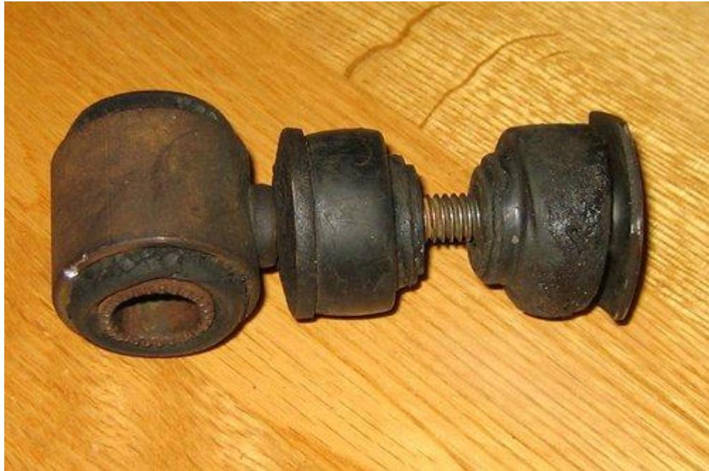
The rear sway bar end links are apparently unique to the II and are next to impossible to find NOS and hard to find in good shape used. Fortunately, there are a few options.
