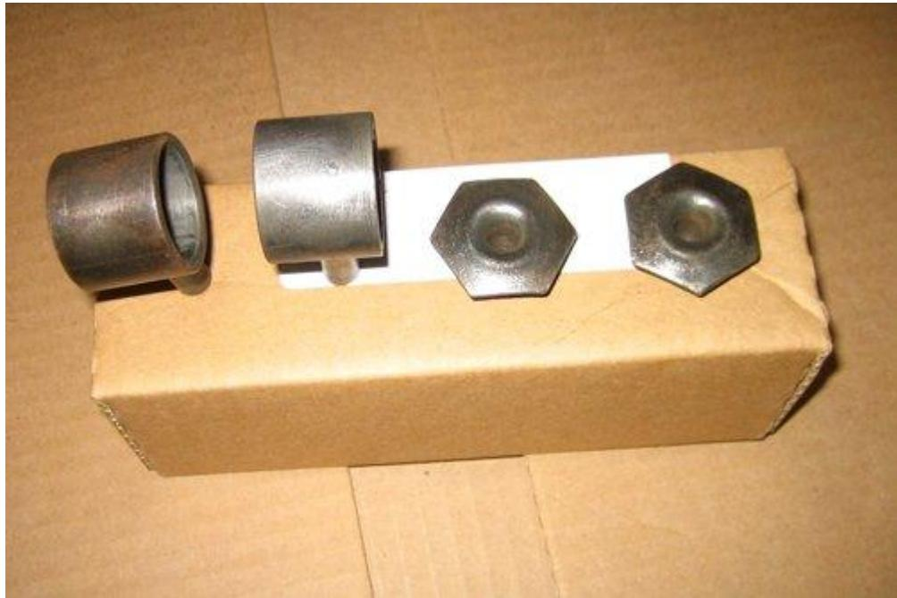
Test fit the bushings into the outer shell and make sure they go in all the way.
